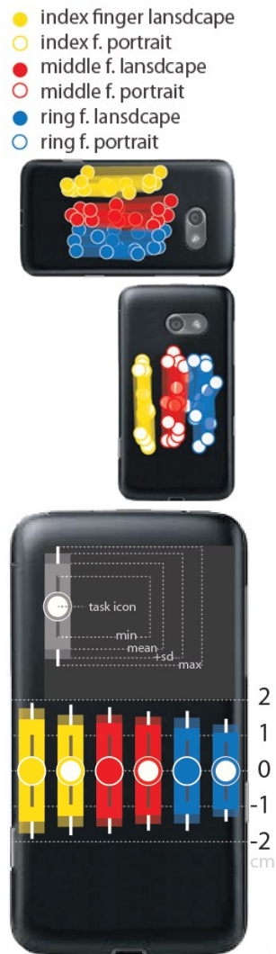
Figure 2. Dragging paths for 3 fingers & 2 device orientations (left), and mean, sd, min, max of dragging lengths (right).
