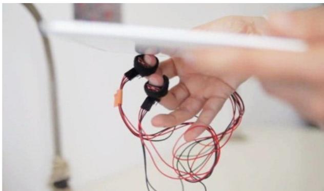
**Figure 2. The prototype that is a fusion board containing an accelerometer, a gyroscope, and a magnetometer detects finger movements.**
