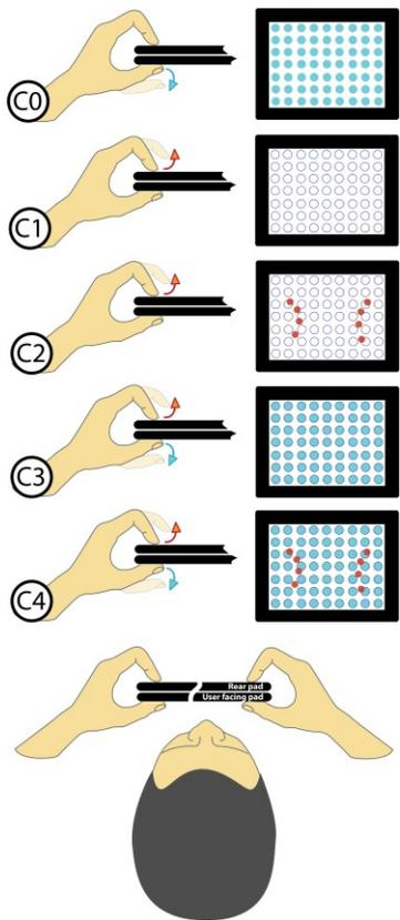
**figure 2** Interactions: participants were asked to select targets by touching and releasing them on different sides of the device. Front only: C0 ●, back only: C1&C2 ○, or both front & back C3&C4 ○. Red circles (●) on the front screen provide feedback about the finger positions at the device's rear in conditions C2 and C4.
