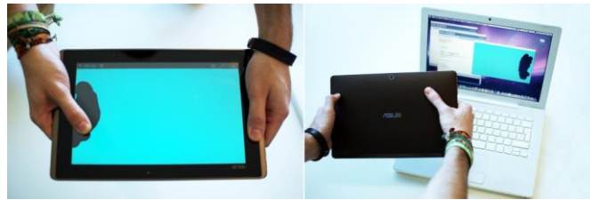
Fig. 1. Apparatus for recording the accessible areas for each thumb and finger.
