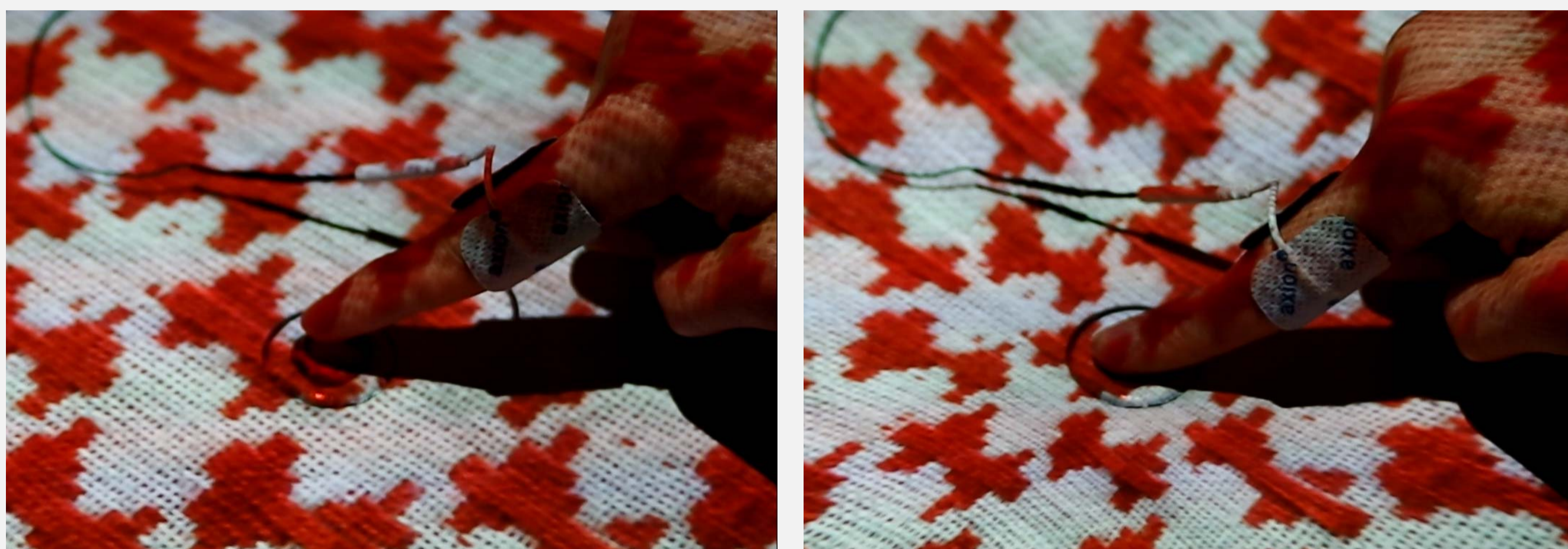
Fig. 1: Texture is projected on a flat metal surface (top) and it is deformed when touched (bottom), which generates the illusion of surface deformation. Additionally or alternatively electro-tactile touch feedback can induce the illusion of touching a deforming surface. Electro-tactile stimuli are generated when touching an electrode embedded into a surface while another electrode is attached to the finger. The apparatus consisted of a TENS device for the electro-tactile feedback, a projector for the visual output, and a pressure sensor underneath the surface to detect the touch/pressure events.
