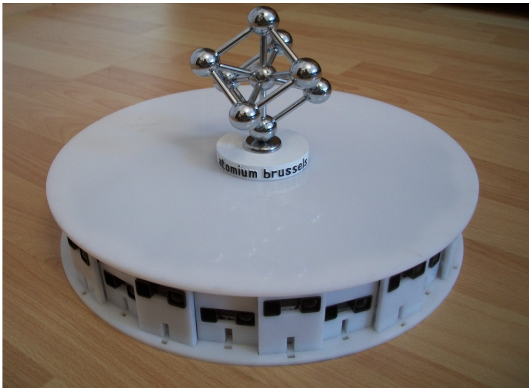
Figure 6: Improved Plinth design using 24 IR sensors to avoid blind spots in sensing proxemics interactions around the Plinth.
