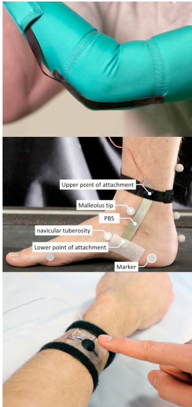
Figure 1 Just some of the different bodily positions stretchable sensors can be worn. Top. elbow angle measurement; middle, gait monitor, and; bottom, skin sensor.
