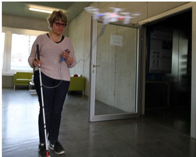
Figure 1: A user is using a leashed quadcopter to navigate in unknown indoor environments. The user can perceive the directions both by hearing the auditory feedback that the quadcopter naturally emits and by feeling the tactile feedback on the handle.
