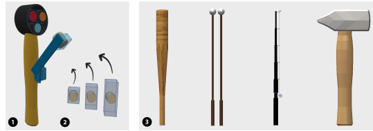
Fig. 6. (1) Concept idea of HapticCollider with interchangeable materials using a revolver cylinder (2) Interchangeable metal weights for HapticCollider (3) Set of interchangeable grips for HapticCollider, grips from left to right: baseball bat, percussion instrument, rod, and hammer.
